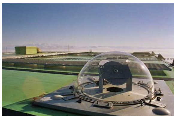
Fig.1 The adjustable mirror system at the Arrival Heights observatory close to Scott Base.
